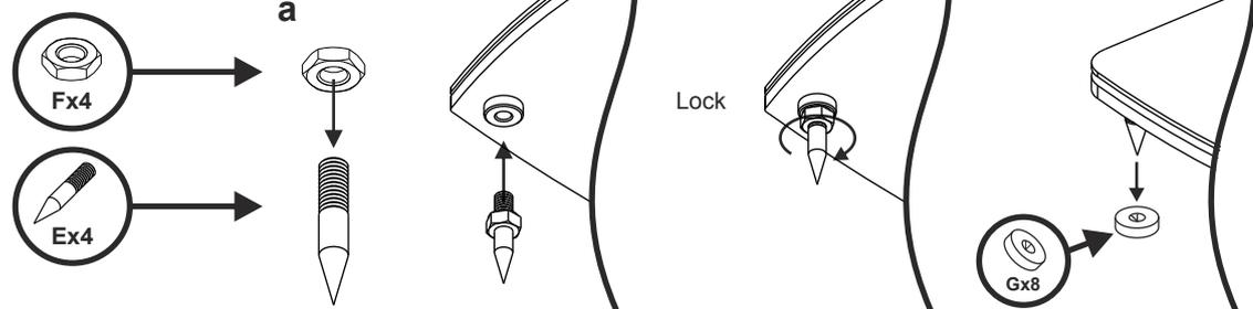
NOTE: In case you have a sensitive floor surface (like hardwood or tiles) which could be damaged by the spikes, please use the spike plates included in the kit (G)
