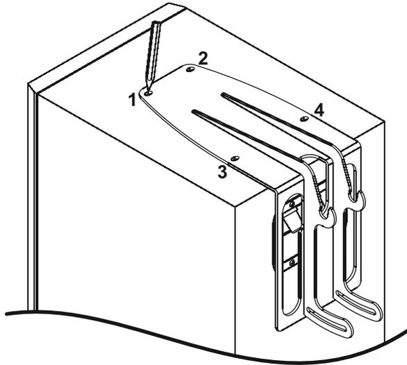
**b** Drill 4 pilot holes in marked positions using drill supplied. Drill to a depth no greater than 15mm.
