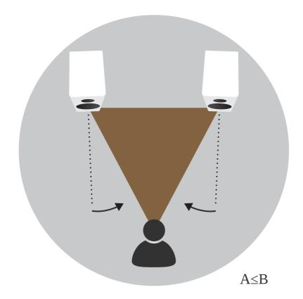
Depending on your personal listening environment and room dimensions, the loudspeakers may be angled in towards the listening area to focus the sound radiation. This positioning will typically improve imaging and is especially recommended by Dynaudio. However, you are free to select the precise position based on your personal listening habits.
