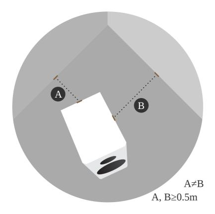
Every loudspeaker not only disperses sound energy directly into the room, but also to the side and even backwards. As a result, time-delayed reflections occur and add to the original music signal. Thus, when loudspeakers are positioned too close to walls, the sound quality can be restricted. Focus XD loudspeakers were developed to be placed free-standing, and therefore they reach their optimum performance when positioned as clear of any walls as possible.
